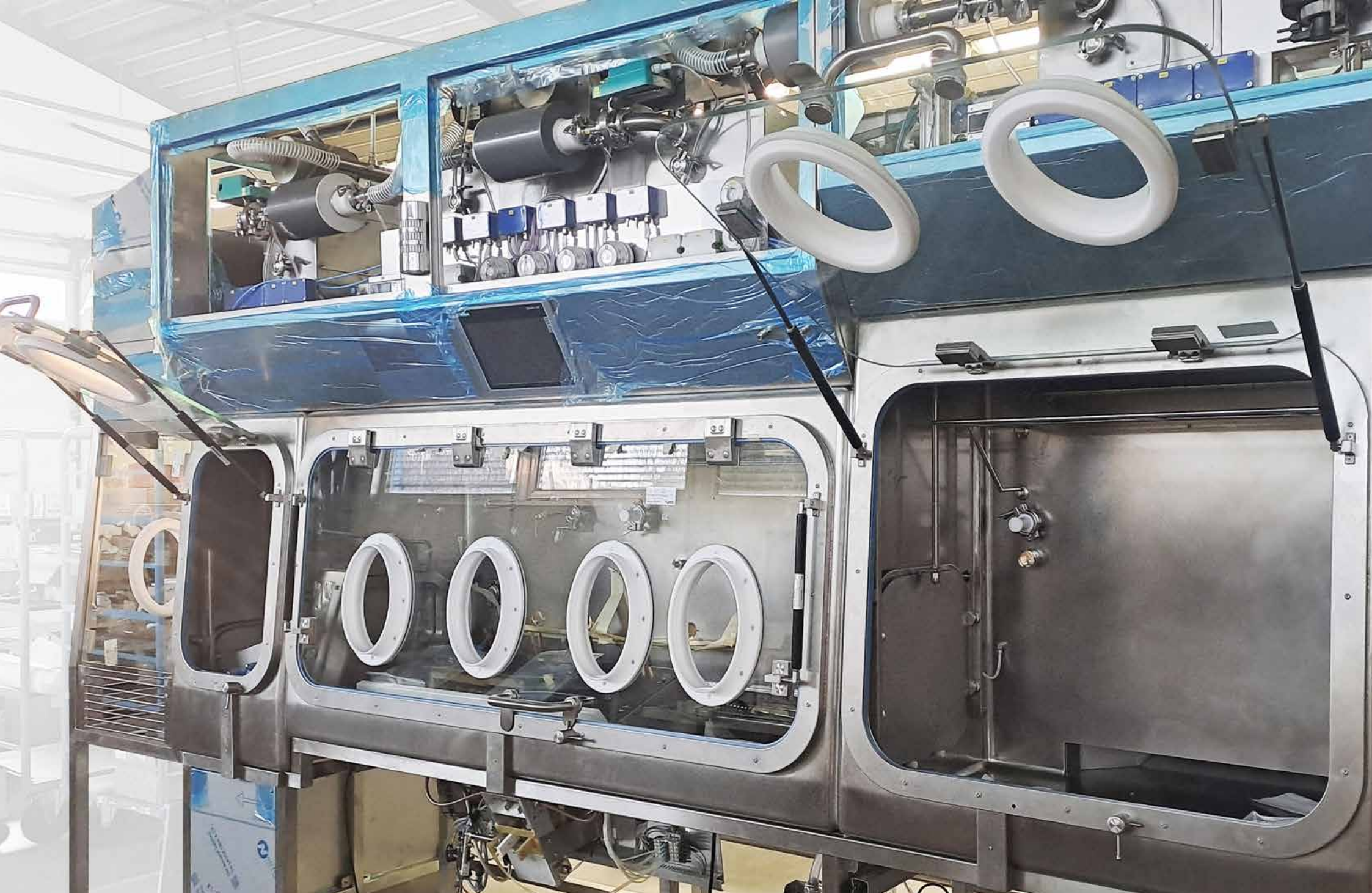
Aseptic Filling Isolator | Carnamedica | Poland
