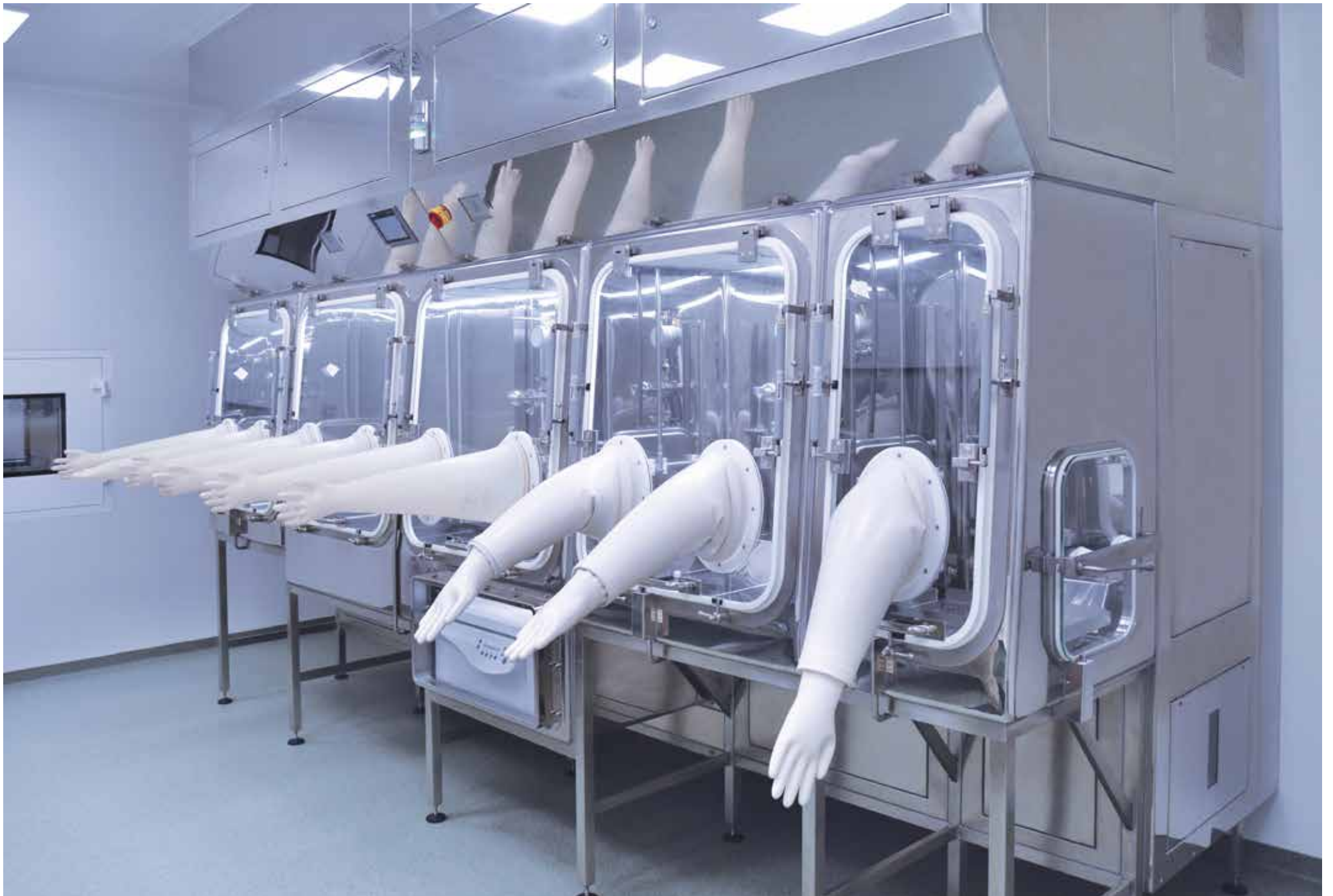
Isolator technology for working with mammalian cells and tissues | Bioceltix S.A. | Wrocław, Poland
